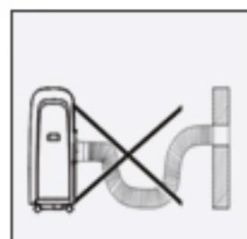
**Keep the air hose as short and free of curves as possible to avoid bottlenecks. The exhaust hose should be no longer than 1,5 meters.**
